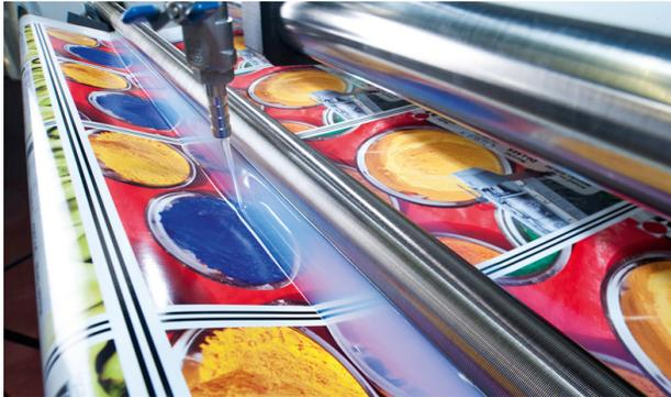
The StarLam 1600R Roll-to-Roll Liquid Laminator applies a smooth, consistent coating of our water-based ClearShield Liquid Coatings, making protecting your digital prints a quick & simple process. The StarLam handles a variety of substrates up to 64" wide, and with our various ClearShield formulations, you will find the perfect coating solution for your application. Our innovative and proven system offers a cost effective laminating solution.
